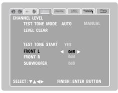
Use the  $\blacktriangle$  and  $\blacktriangledown$  cursor buttons to select the speaker from which the test tone is to be output, then use the  $\blacktriangleleft$  and  $\triangleright$  cursor buttons to adjust the channel levels so that the volume of the test tones output from the different speakers sounds the same.
